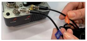
The antenna is extended to the roof of the vehicle and fixed to it using the magnet that is on the bottom of the antenna. If the antenna is not mounted to the roof of the vehicle only the connectors are attached.
