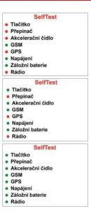
If everything is in order, the Self-test takes 38 seconds. If something is not in order, the Self-test automatically ends after 2 minutes and shows error. The results of the Self-test are sent to the server where records are available for viewing
